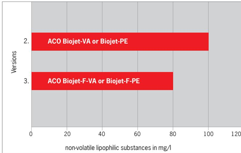
The levels of non-volatile lipophilic substances can be reduced by implementing the treatment process.
