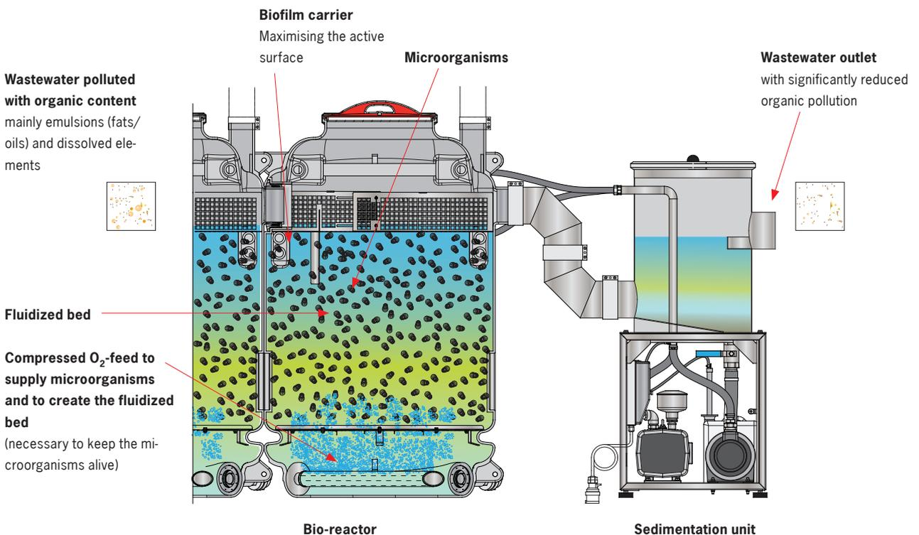
By using the new ACO Biojet a significant reduction of pollution levels (non-volatile lipophilic substances) is achieved. This means that it is possible to comply with the pollution threshold imposed by many local authorities of 100 mg/l of non-volatile lipophilic substances. Here too, all that is required are normal working conditions and proper procedures as set out in DIN 4040-100.
