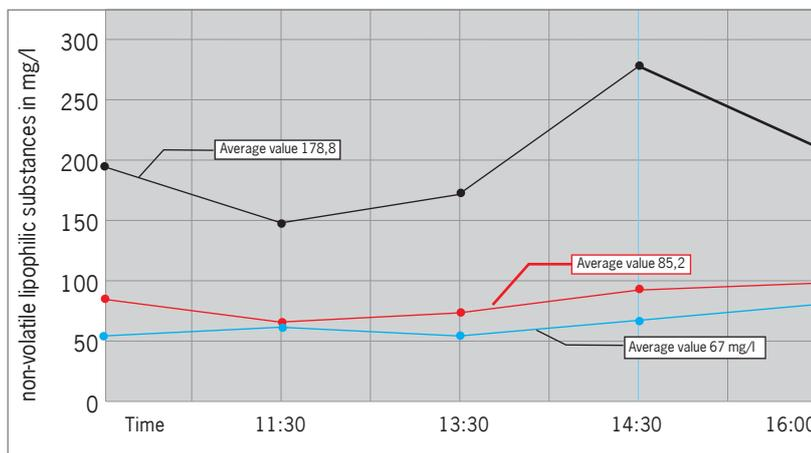
For example this diagram shows the values measured from an ACO Building Drainage treatment plant consisting of a grease separator, a biological unit and a sedimentation and filtration unit.
