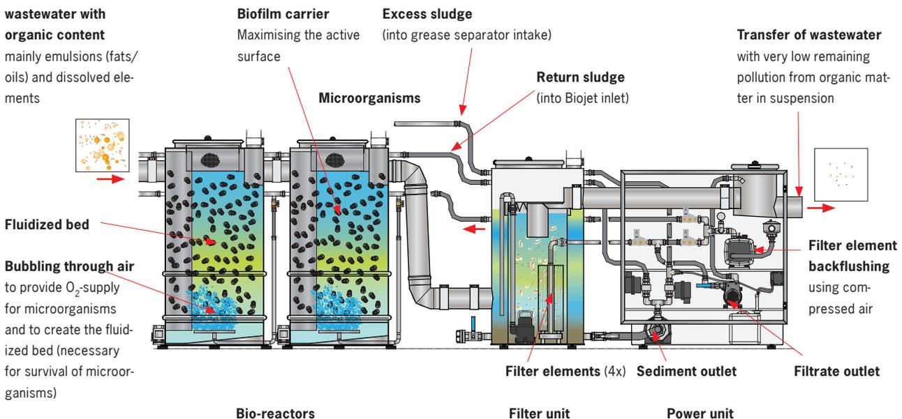
By using the new ACO Biojet-F a significant reduction in pollution levels (non-volatile lipophilic substances) is achieved. This means that it is possible to comply with the pollution threshold imposed by many local authorities of 80 mg/l of non-volatile lipophilic substances. Here too, all that is required are normal working conditions and proper procedures as set out in DIN 4040-100.
