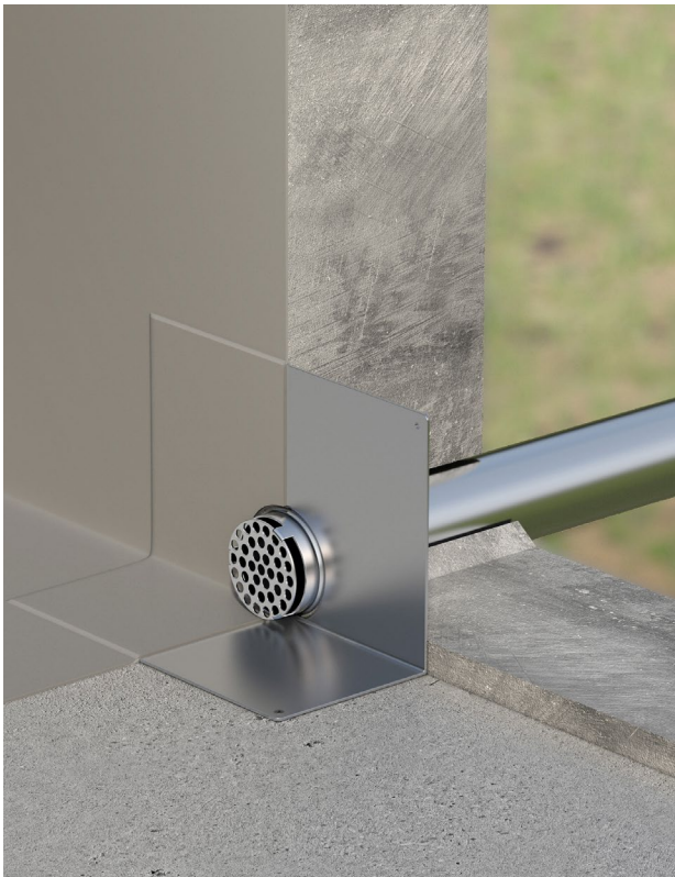
ACO spout for main drainage - flush with the balcony slab, sealed with liquid plastic sealant.
