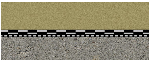
Balcony with waterproofing membrane, reversed roof
