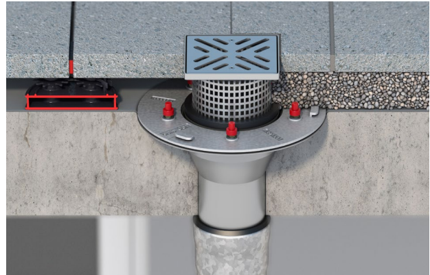
Balcony drain with compression seal flange for installation in a balcony slab with waterproofing membrane and additional covering surface
