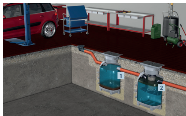
1 Sludge trap 2 Coalisator-P light oil separator
